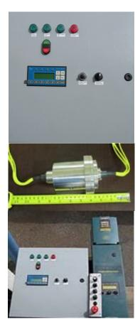
Baldor MICROdrive provides, variable torque, constant torque or constant horsepower and features Volts per Hertz Control with peak overload capacity of 175%.
