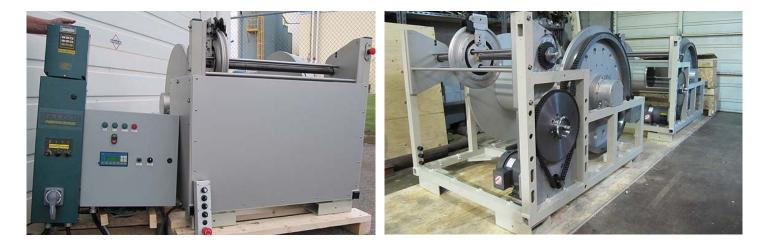
**Structure**—Welded Aluminum, compact, weigh less and DNV 2.7-3 compliant. **Safety** - Winches are safer for both Operators and Equipment, cable is enclosed inside the cover, have 3 (three) E-Stop Buttons, 2 (two) Safety Clutches, Mechanical or Electrical Brakes.
